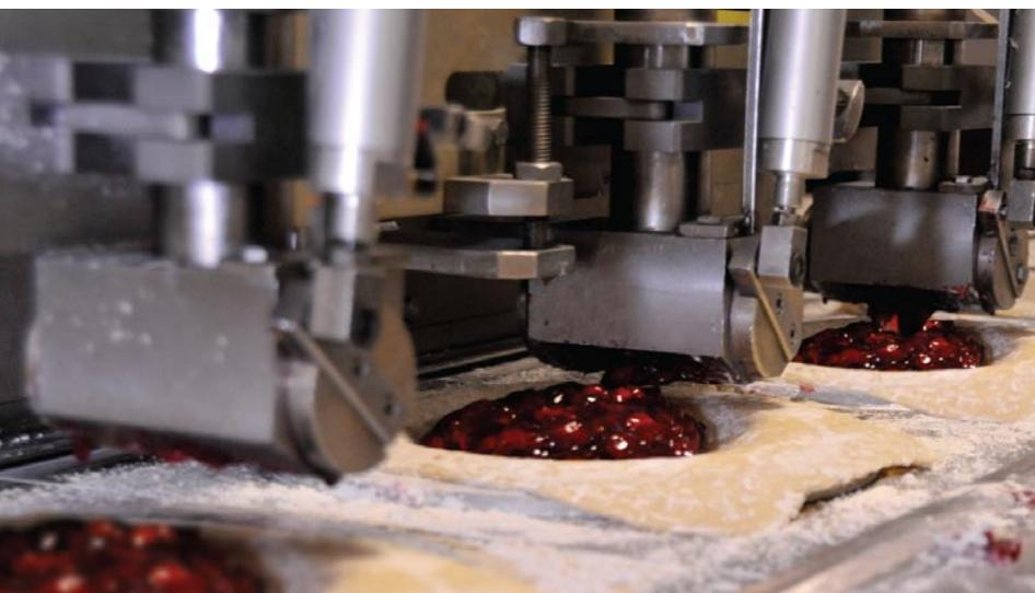
Cherry filling is automatically deposited into pie crusts.
